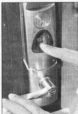
This electronic device opens a door if it recognizes certain approved fingerprints.
